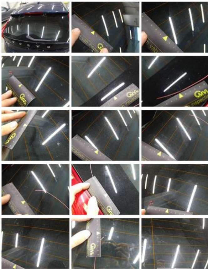
Roof, Chemical polution, LI - Repair and paint (complete)
