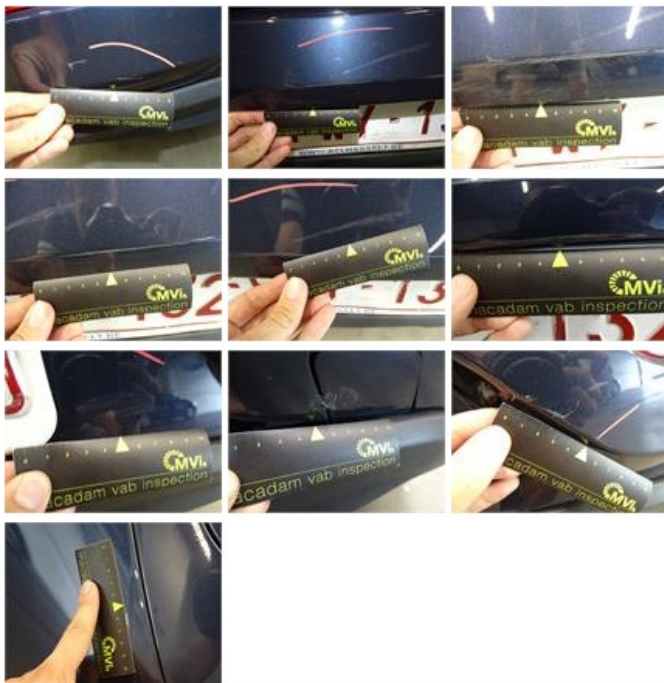
Bonnet, Chemical polution, LI - Repair and paint (complete)
