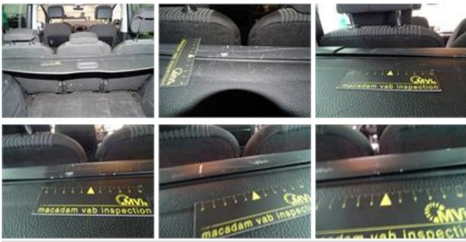
Sidewall panel RL, Broken, E - Replace
