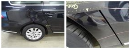
Door frame F L, Dent(s), It - Spot repair
