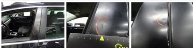
Backrest cover F L, Damaged, E - Replace
