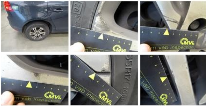
Door moulding Lower R R, Dent(s) and scratch(es), E - Replace
