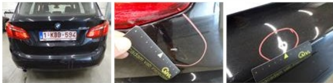
Rearlight R , Broken, E - Replace
