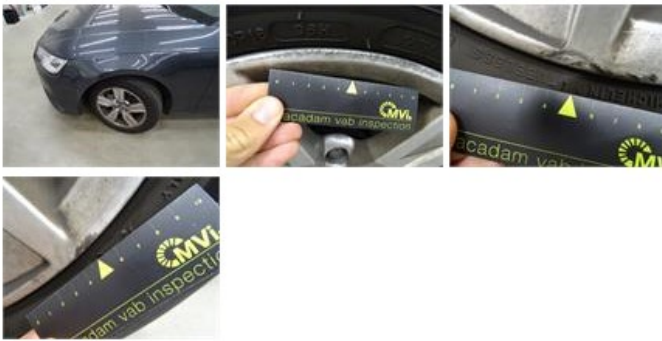
Bumper R, Crack, Le - Replace and paint
