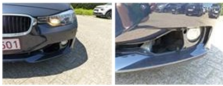
Bumper grille F R, Broken, E - Replace
