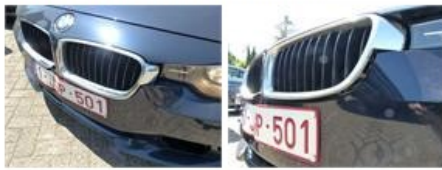
Bumper grille F L, Broken, E - Replace
