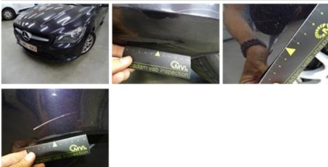
Door F L, Bad repair, Acceptable
