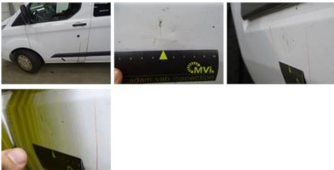
Sidewall RL (LCV), Dent(s), It - Spot repair
