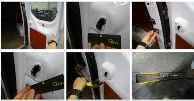
Trunk door R L, Dent(s) and scratch(es), It - Spot repair
