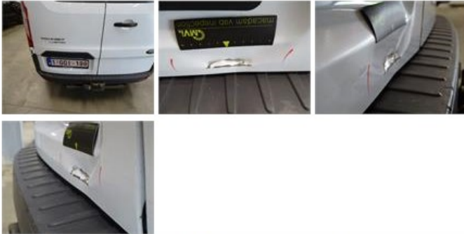
Wing F R, Deformed / Strained, LI - Repair and paint (complete)
