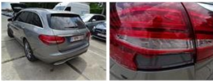
Rearlight L, Broken, E - Replace
