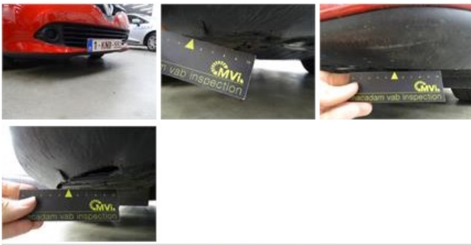
Wing R R, Scratch(es), LI - Repair and paint (complete) 246,56
