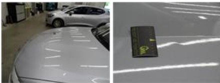
Bonnet, Dent(s), PDR - Paintless dent repair
