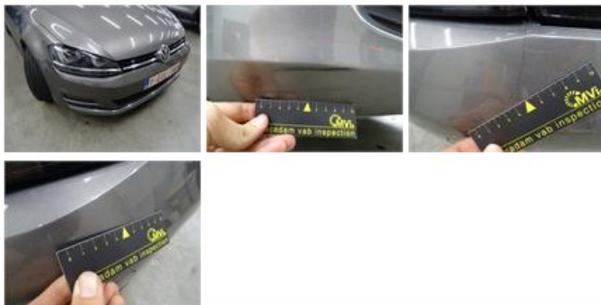
Sill outer L, Dent(s) and scratch(es), LI - Repair and paint (complete)
