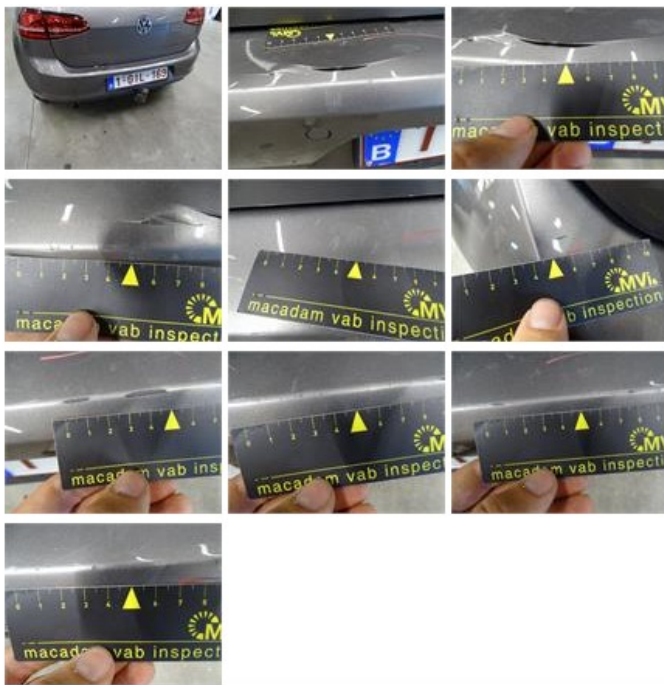
Bumper F, Crack, Le - Replace and paint
