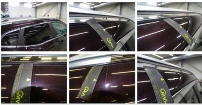
Roof pillar L, Hail damage, PDR - Hail
