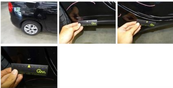
Wing F L, Dent(s) and scratch(es), LI - Repair and paint (complete)
