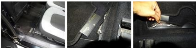
Rocker panel inner R L, Scratch(es), Acceptable
