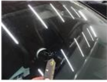
Windscreen, Stone chip(s), Windscreen repair
