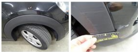
Bumper moulding F, Scratch(es), E - Replace
