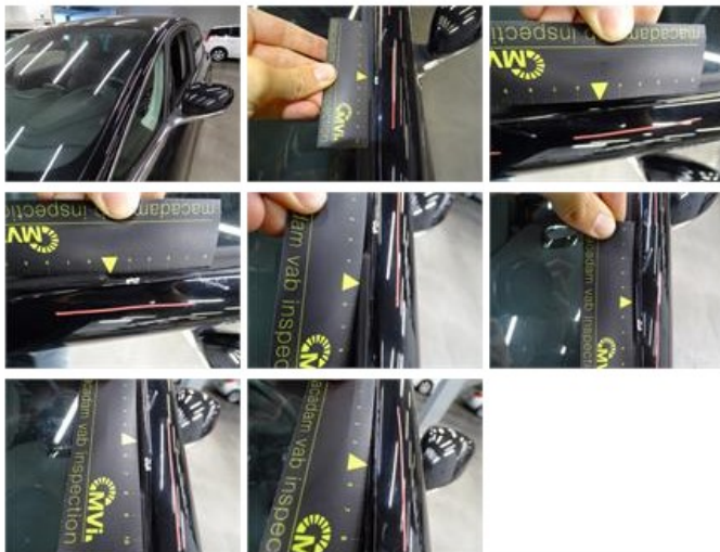
Trunk lid covering R, Scratch(es), Acceptable
