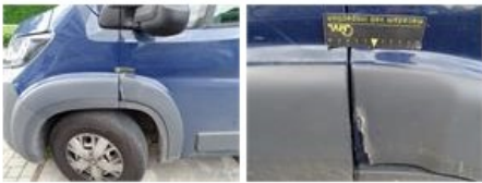
Wing moulding F L, Broken, E - Replace
