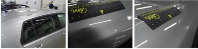
Door R L, Bad repair, Acceptable
