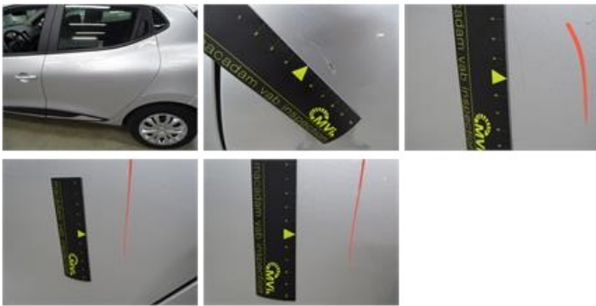
Rear window, Scratch(es), Acceptable
