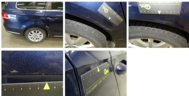
Wing F L, Dent(s) and scratch(es), LI - Repair and paint (complete)
