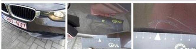
Bumper F, Dent(s) and scratch(es), Le - Replace and paint
