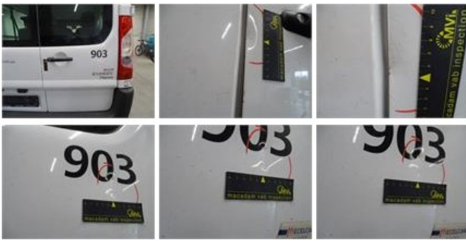
Sill outer R, Dent(s) and scratch(es), LI - Repair and paint (complete)
