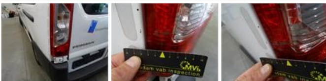
Bumper grille, Deformed / Strained, E - Replace
