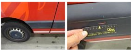
Door R R, Dent(s), LI - Repair and paint (complete)
