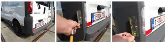
Trunk door R L, Dent(s) and scratch(es), LI - Repair and paint (complete)
