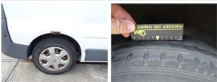
Wheel cover R L, Missing, E - Replace
