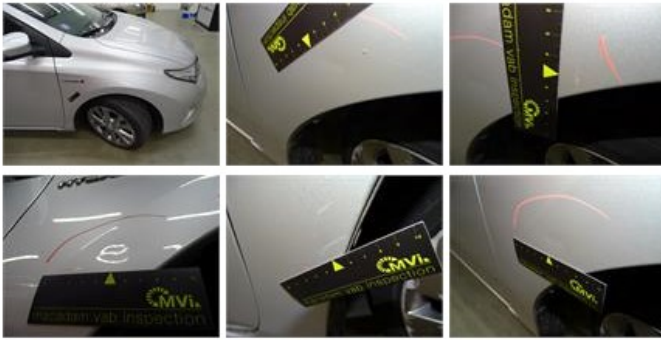
Spoiler R, Dent(s) and scratch(es), It - Spot repair
