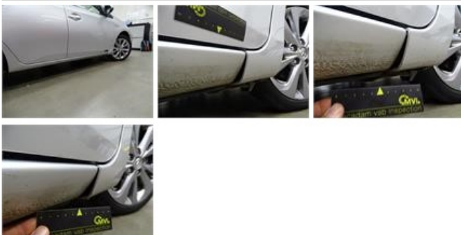
Door F L, Dent(s) and scratch(es), LI - Repair and paint (complete)
