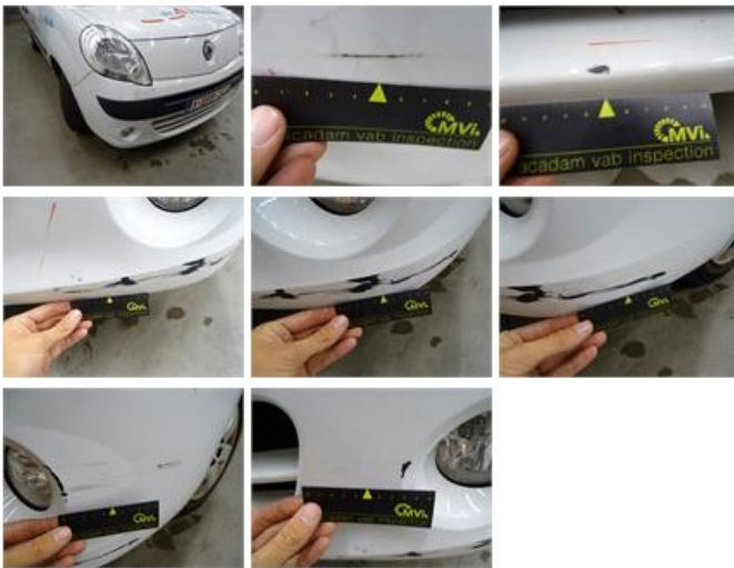
Wheel cover F R, Deformed / Strained, E - Replace
