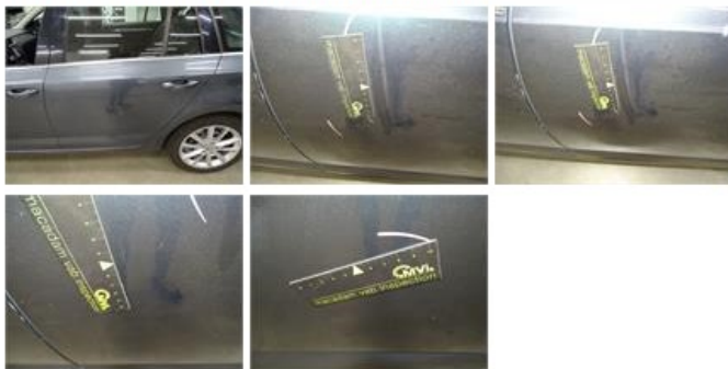
Sidewall panel RL, Missing, E - Replace
