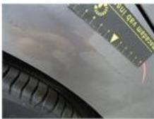
Tailgate, Dent(s) and scratch(es), LI - Repair and paint (complete)
