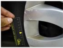
Wheel cover F L, Scratch(es), E - Replace
