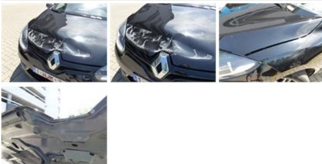
Bumper grille F R, Deformed / Strained, E - Replace
