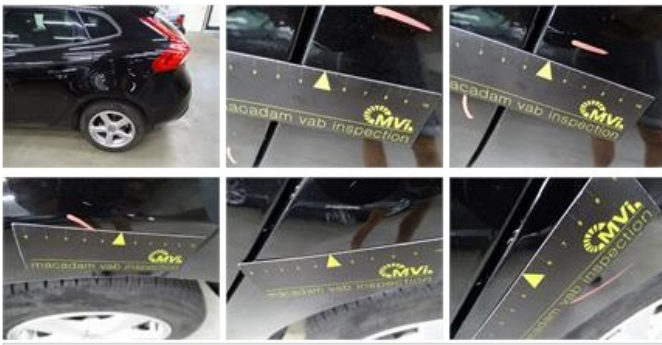
Tailgate, Scratch(es), LI - Repair and paint (complete)
