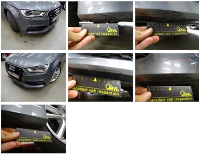
Spoiler R, Scratch(es), LI - Repair and paint (complete) 115,56
