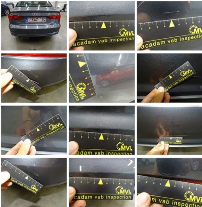
Sill outer R, Deformed / Strained, Le - Replace and paint
