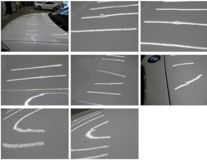
Roof, Hail damage, PDR - Hail
