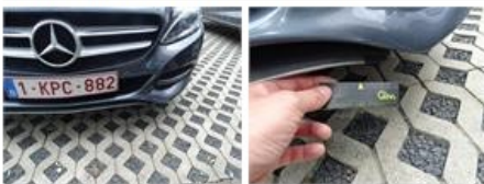
Bumper moulding F, Broken, E - Replace
