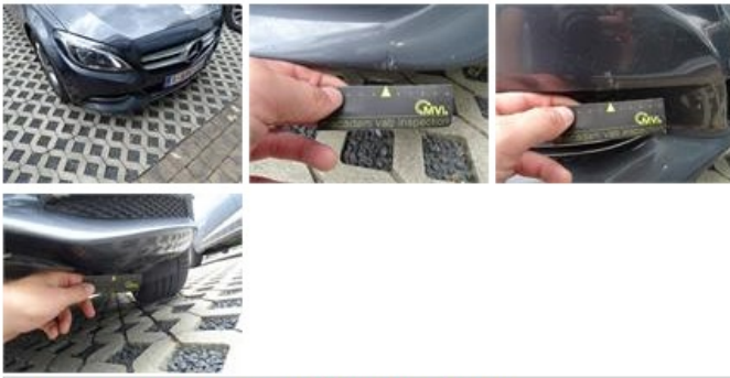
Sill outer L, Scratch(es), LI - Repair and paint (complete)
