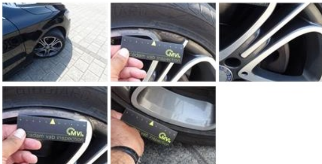
Alloy rim R R polished, Scratch(es), LI - Repair and paint (complete)
