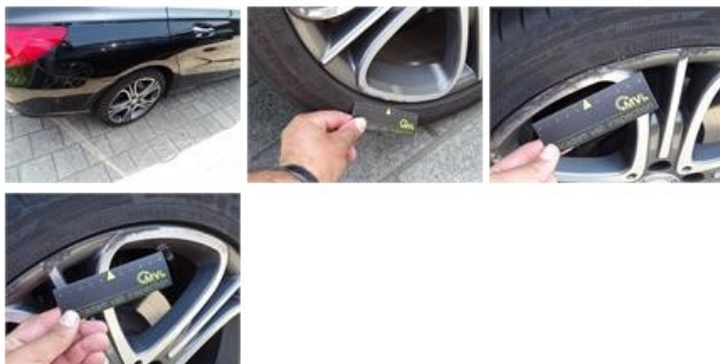
Alloy rim R R polished, Scratch(es), LI - Repair and paint (complete)
