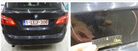
Wing F L, Chemical polution, LI - Repair and paint (complete)
