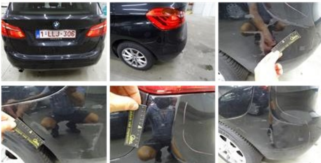
Tailgate, Scratch(es), LI - Repair and paint (complete)
