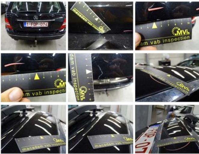
Roof, Chemical polution, LI - Repair and paint (complete)
