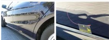
Roof pillar R, Dent(s), Acceptable
