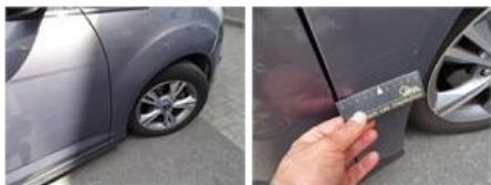
Door panel F L, Scratch(es), Acceptable
