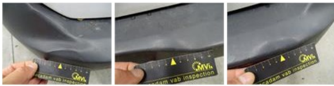
Trunk door R R, Dent(s) and scratch(es), It - Spot repair
