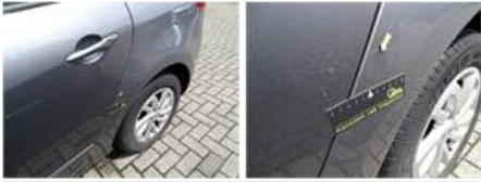
Sill outer R, Dent(s), It - Spot repair
