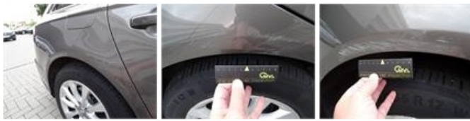
Wing F R, Dent(s) and scratch(es), LI - Repair and paint (complete)
