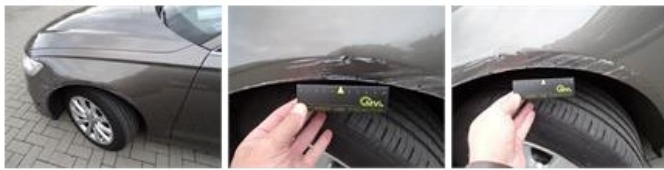
Wing F L, Dent(s) and scratch(es), Le - Replace and paint
