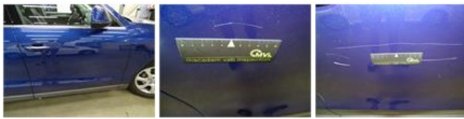
Protection plate M, Deformed / Strained, E - Replace
