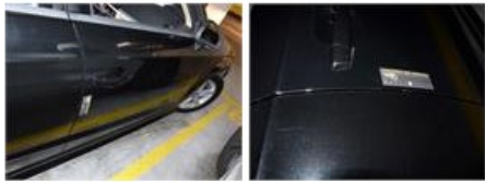
Roof pillar R, Scratch(es), LI - Repair and paint (complete)
