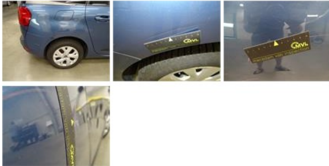
Rocker panel inner R R, Dent(s), LI - Repair and paint (complete)
