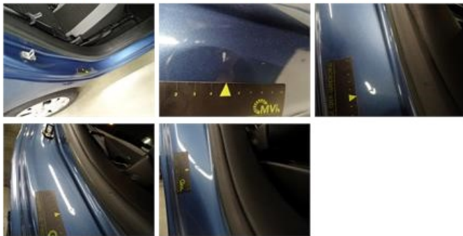
Door R R, Dent(s) and scratch(es), LI - Repair and paint (complete)
