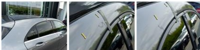
Roof, Scratch(es), LI - Repair and paint (complete)
