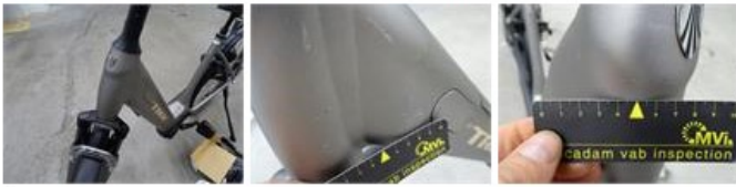
Protection plate M, Deformed / Strained, E - Replace
