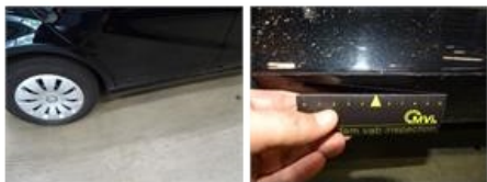
Bumper R, Crack, Le - Replace and paint
